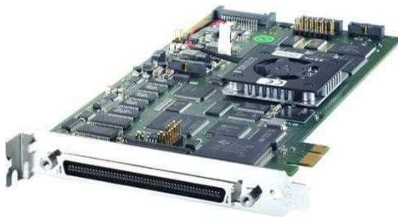
Fig. 3.1.2 Photo of the DS1104 controller board.
